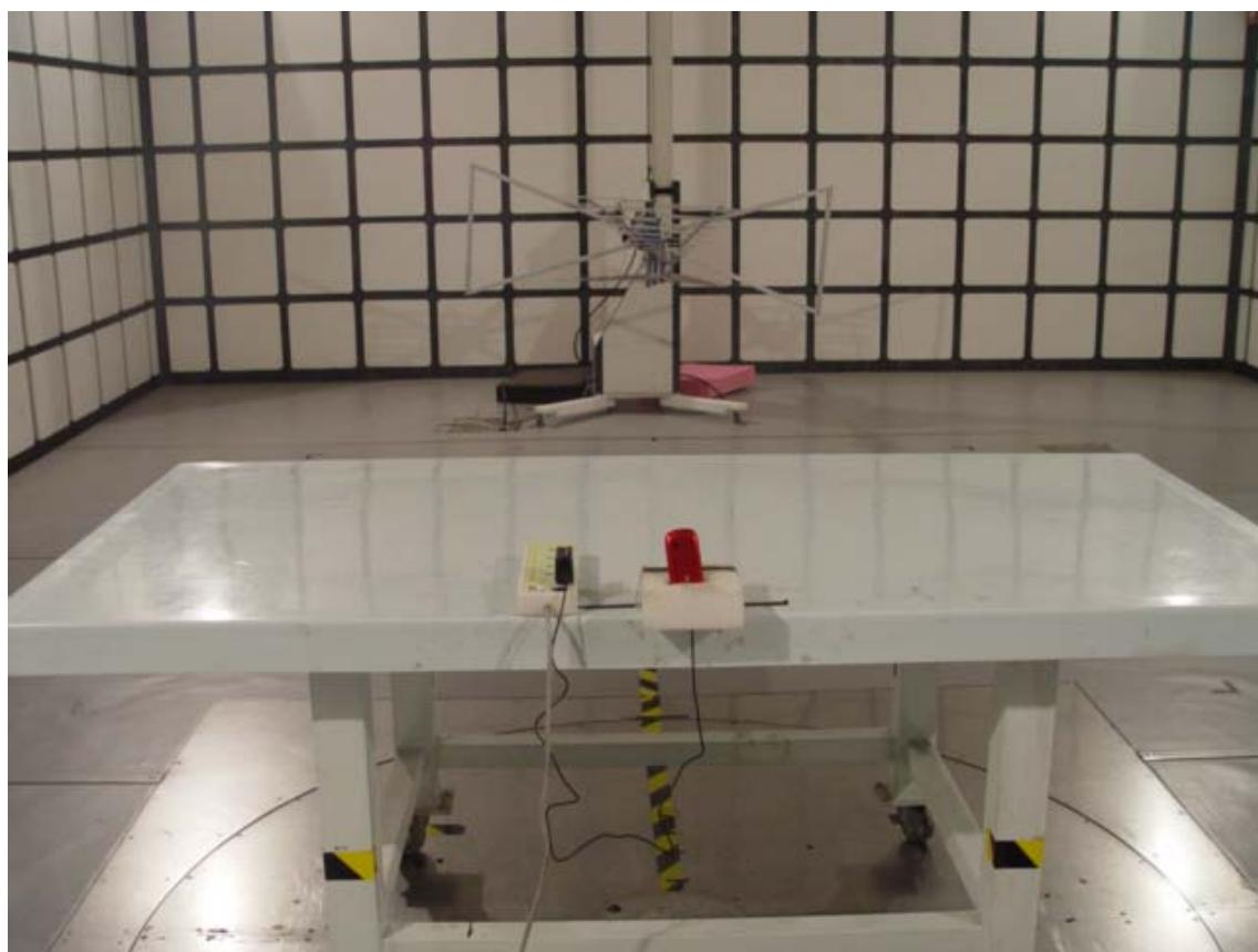
**FCC Part15C Radiated Emission above 1GHz****-Front**
