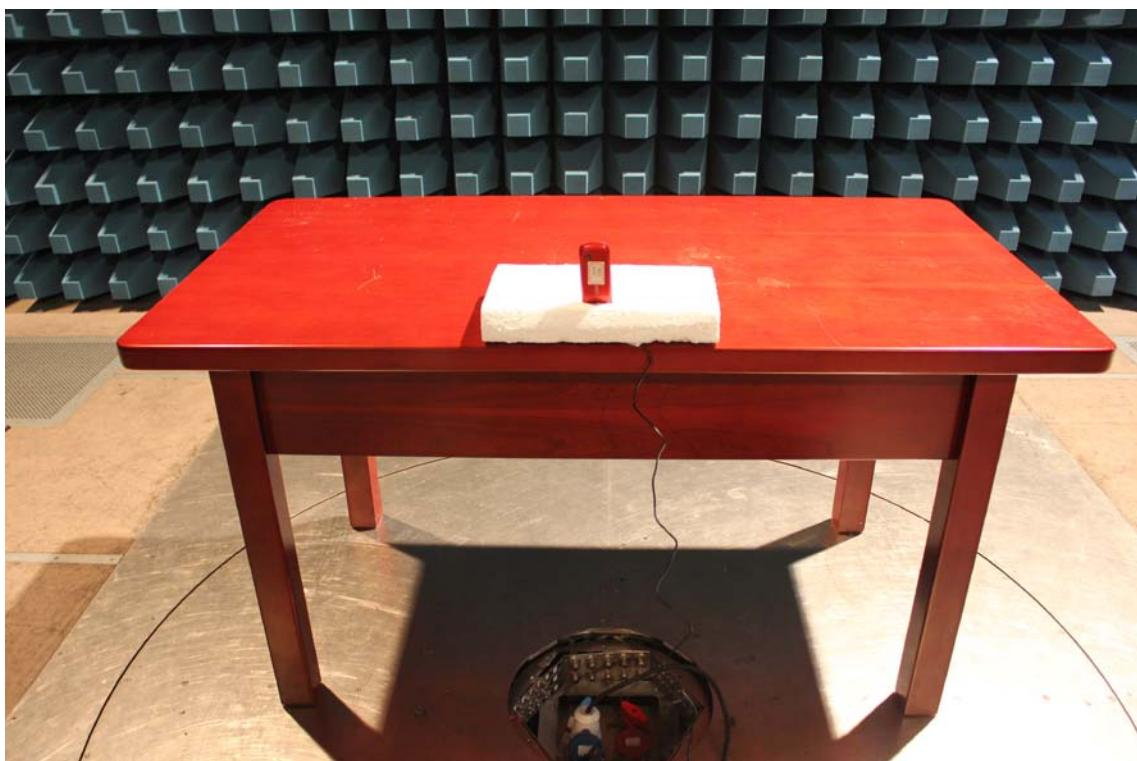
**FCC Part15C Radiated Emission below 1GHz****- Front**
