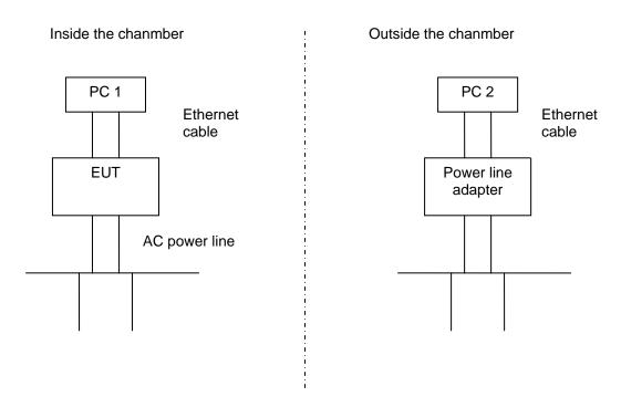
**Equipment Used in Tested System**
