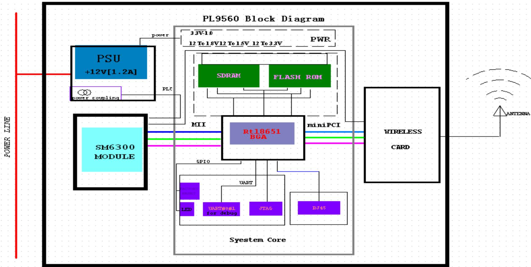
Power line  $\leftrightarrow$  PT2 Powerline network signal coupling  $\leftrightarrow$  SM6300 module implement powerline network signal conversion MII interface Data  $\leftrightarrow$  U1 Rt18651 Controller  $\leftrightarrow$  Determine the modulation type,WLAN Access Point controller  $\leftrightarrow$  Mini PCI interface Transmission and Receive network communications Data  $\leftrightarrow$  Wirless Card RF(2.42-2.484G) signal generator and control Wireless signal
