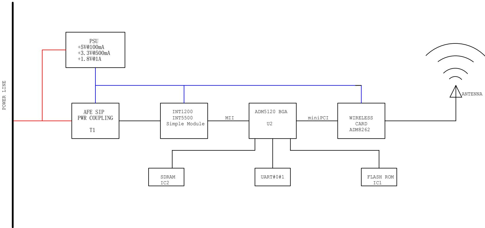
Power line → T1 powerline network signal coupling → Simple module implement powerline network signal conversion MII interface signal → U2 ADM5120 controller → Determine the modulation type , WLAN access point controller → Mini PCI interface send out transmission signal → Wireless Card RF(2.412-2.484G) signal generator and control → Antenna transmit signal out from Antenna
