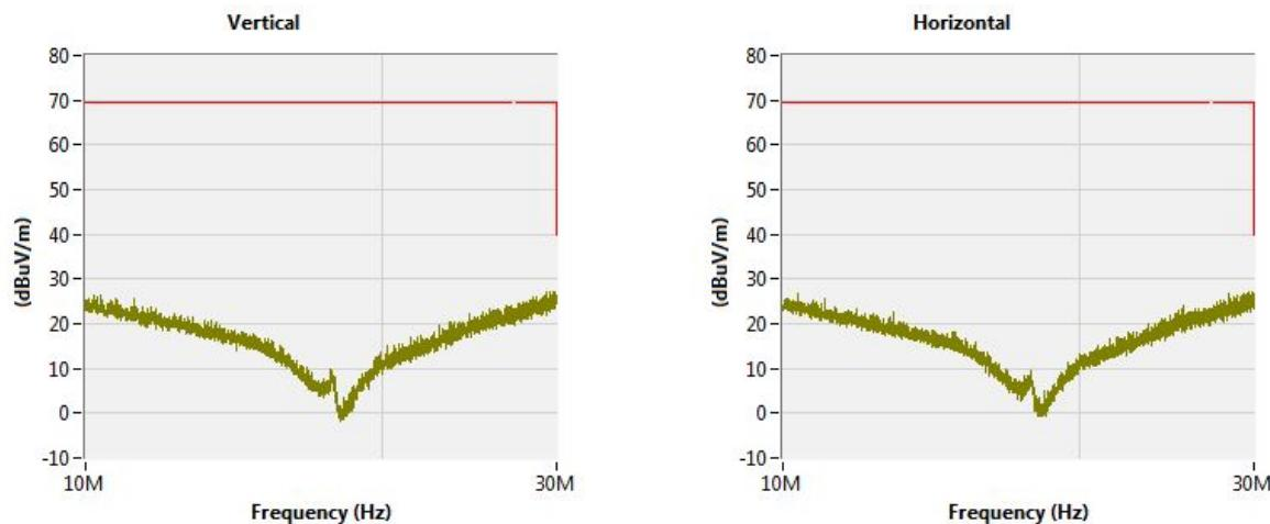
Scan shows only ambient noise floor from 10 to 30MHz.
