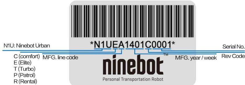
Figure 5: Serial number label and code explanation
