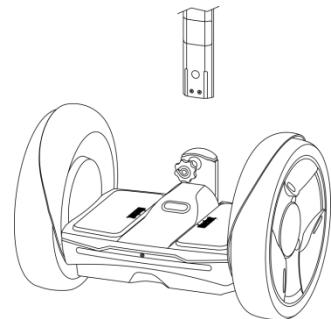
Figure 7: Mount the Operation Bar to the Mainframe.
