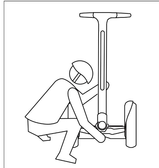
Figure 36: Deploying the parking stand
