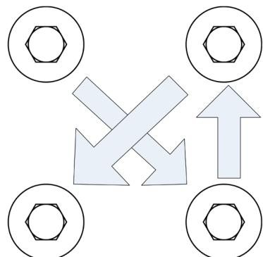
Figure 41: Tighten in a Cross Pattern
