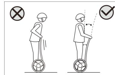
Figure 13: Do not lean against the Operation Bar.
