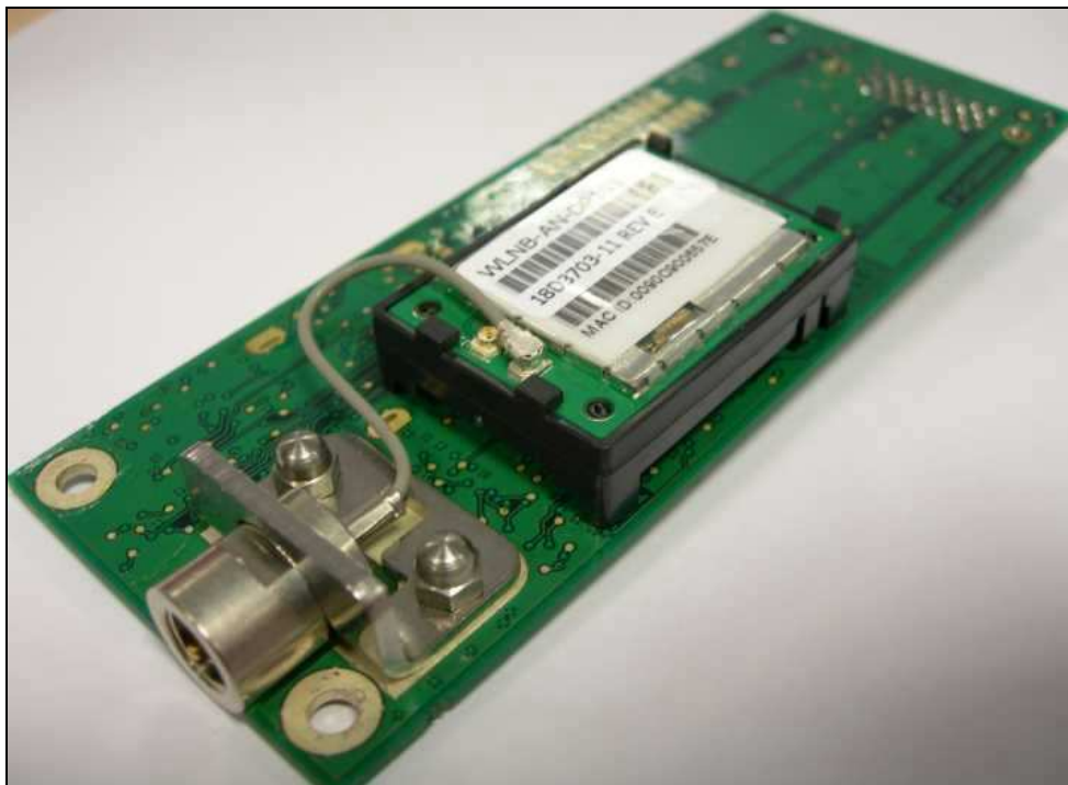
MODEM DAUGHTER BOARD (TOP & BOTTOM VIEW) + MODEM DPAC WLNb-AN-DP101
