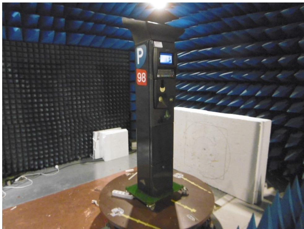
Anechoic chamber setup
