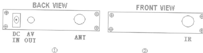
4. Connect the power transformer (7V/500mA) to the camera (Battery of the same voltage is acceptable).
