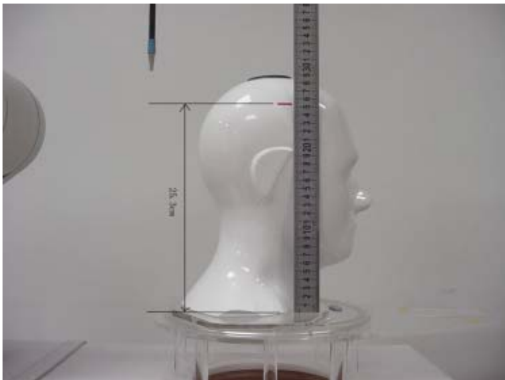
Fig.2 The depth of head tissue in SAM
