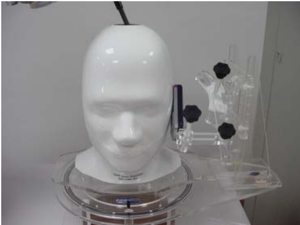
Fig.3 EUT Left Head Touch Cheek Position
