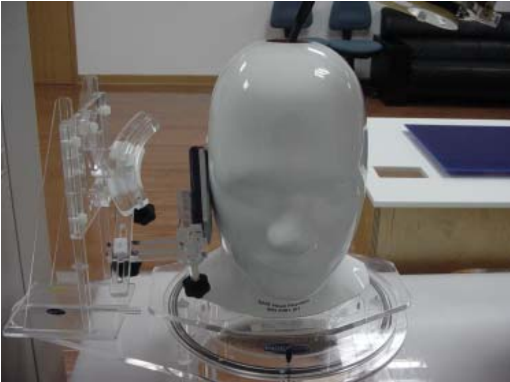
Fig.5 EUT Right Head Touch Cheek Position
