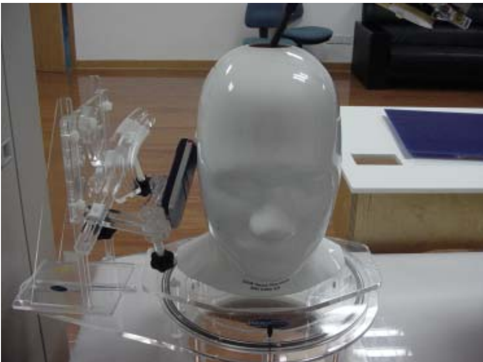
Fig.6 EUT Right Head Tilt15 Position
