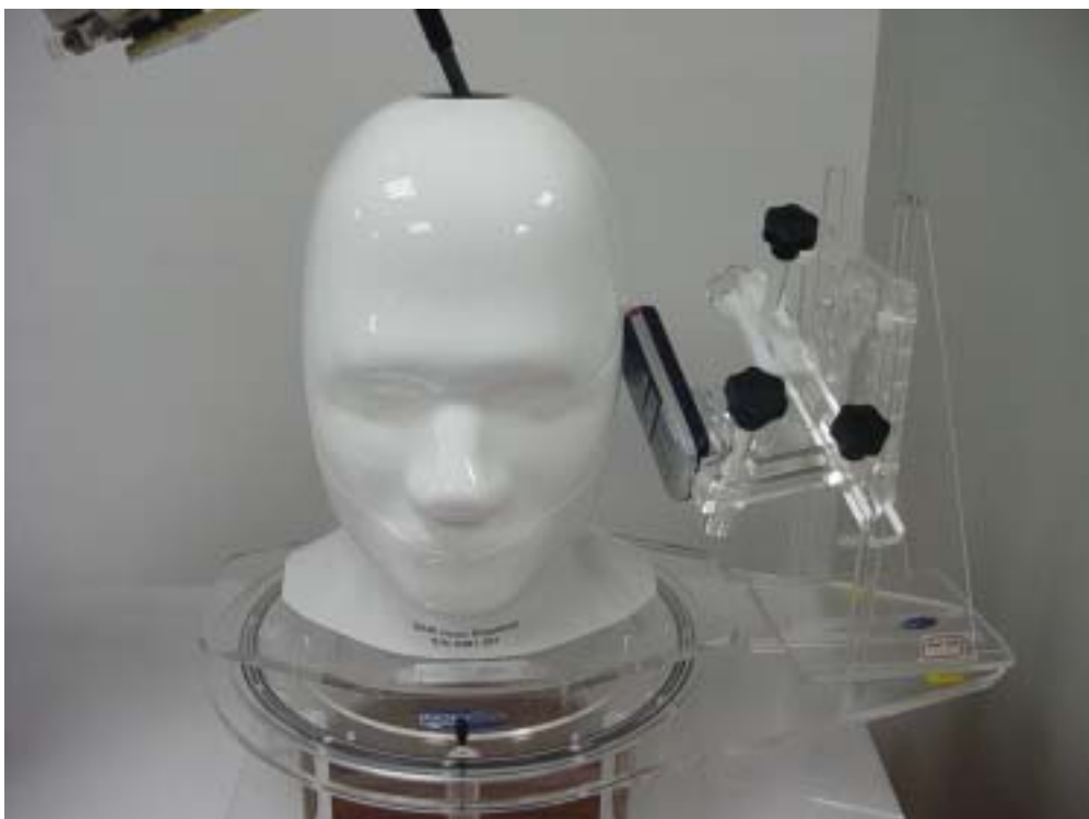
Fig.4 EUT Left Head Tilt15 Position
