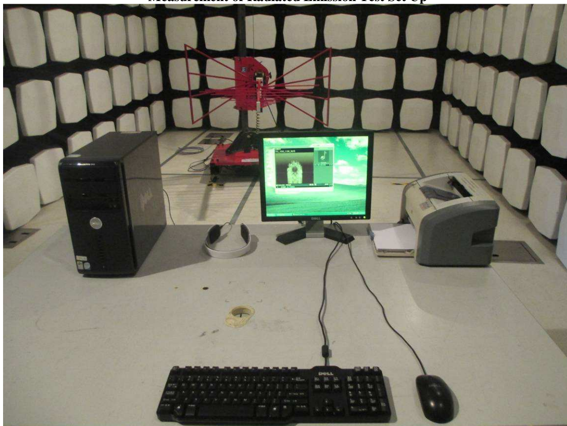
Measurement of Radiated Emission Test Set Up
