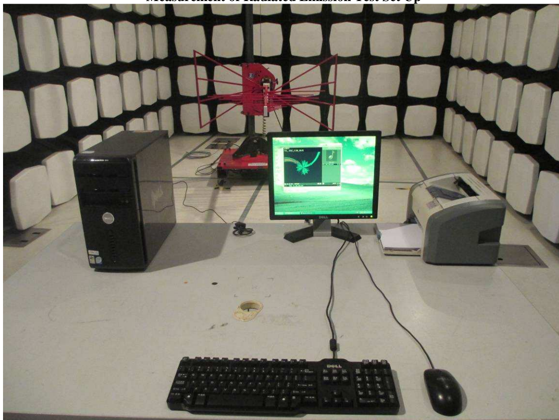
Measurement of Radiated Emission Test Set Up
