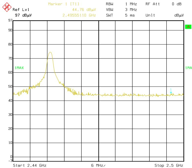
**Band Edge Left Side - Vertical**
