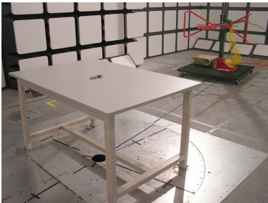
Radiated Emission - Rear View (30-1000MHz)
