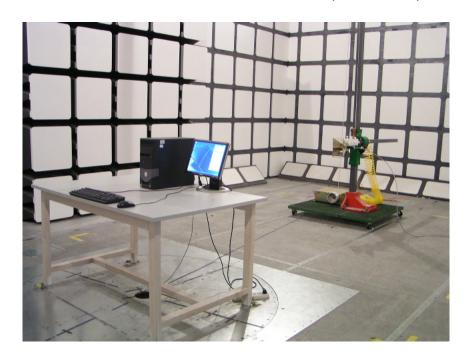
Radiated Emissions – Rear View for Base (Above 1GHz)
