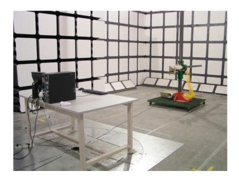
Radiated Emissions - Front View for Handset (30 MHz-1000MHz)
