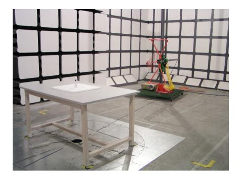
Radiated Emissions - Rear View for Handset (30 MHz-1000MHz)
