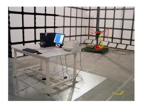
Radiated Emissions - Rear View for Base (30 MHz-1000MHz)
