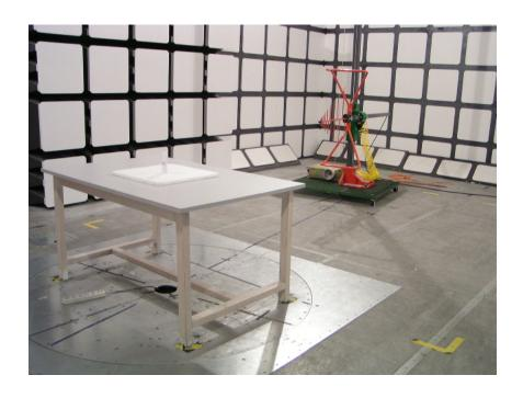
Radiated Emissions – Front View for Handset (Above 1GHz)
