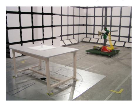
**Radiated Emissions – Rear View for Handset (Above 1GHz)**
