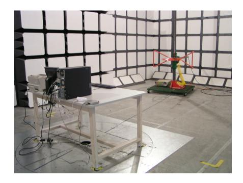
Radiated Emissions – Front View for Base (Above 1GHz)
