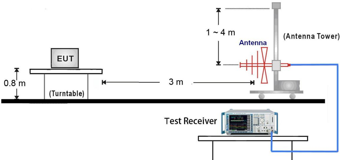
1GHz ~ 18GHz Test Setup:
