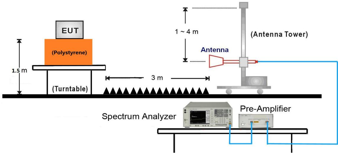
18GHz ~25GHz Test Setup:
