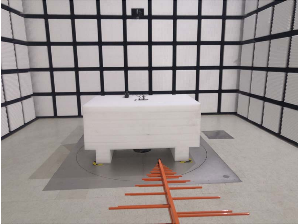
Radiated Emissions Below 1G front View
