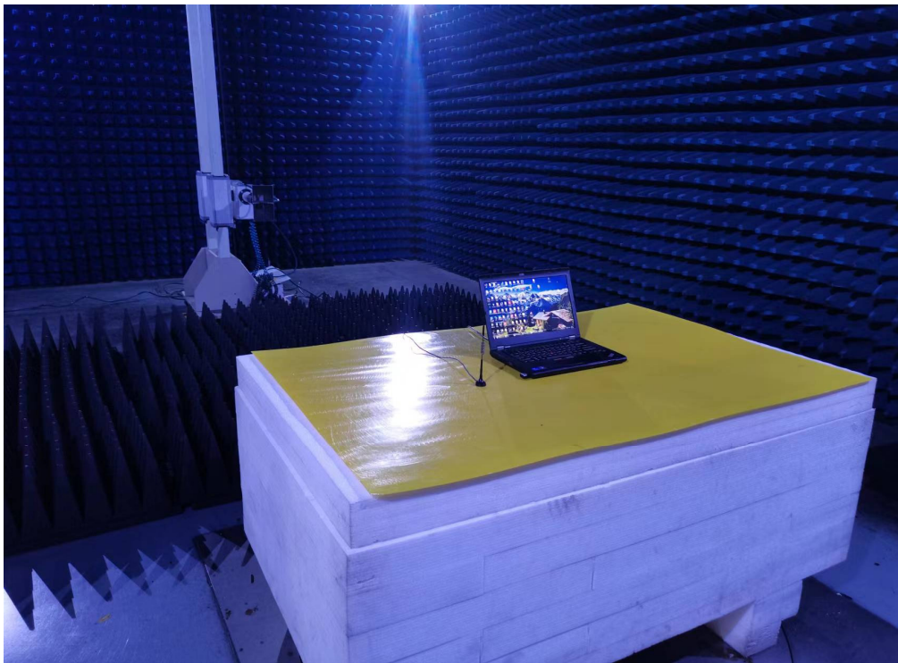
Photo of Radiated Emission Measurement (Above 1G)
