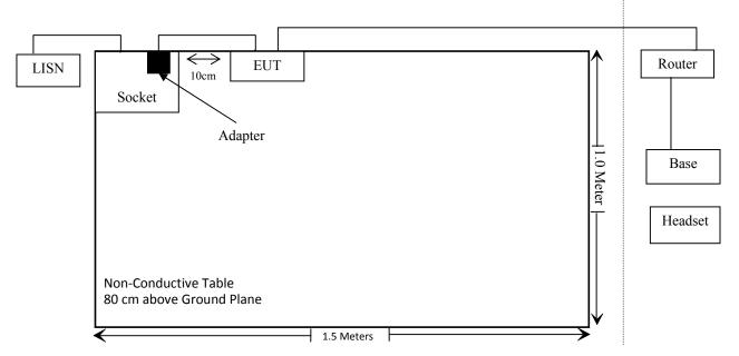
Test Mode2: TX (Powered By POE)
