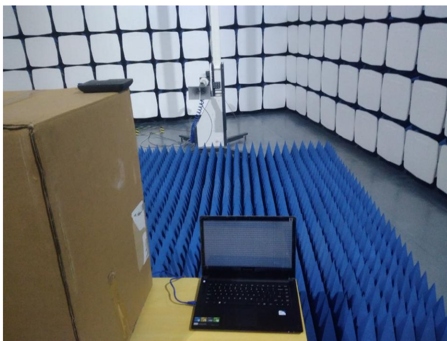
FP - Radiated Emission test view (Frequency above 1GHz)
