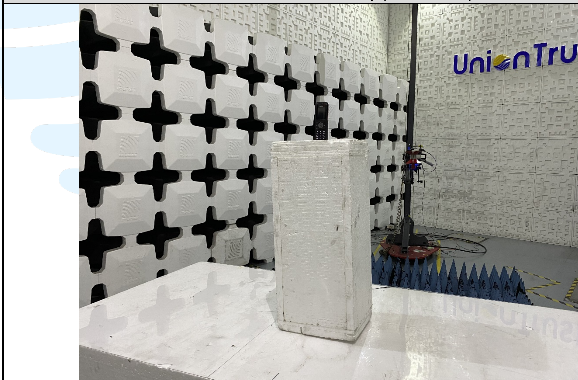
Radiated emission Test Setup (Above 1 GHz)
