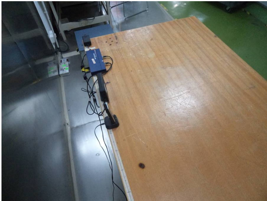
Conducted Emissions - Side View (PoE power)
