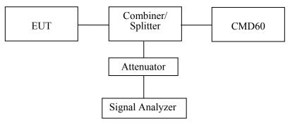
The width, in Hz, of the signal between two points, one below the carrier center frequency and one above the carrier center frequency, that is 26 dB down relative to the maximum level of the modulated carrier. It is based on the use of measurement instrumentation employing a peak detector function with an instrument resolution bandwidth approximately equal to 1% of the emission band-width of the device under measurement. [Extraction from 47 VFR 15, subpart D, 15.303 (C)].
