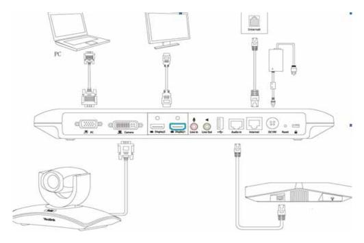
1. (Optional) The use of screw Camera is fixed on the wall bracket, and the DVI at the other end of the line is connected to the Camera interface on the  $VC400\ host.$
