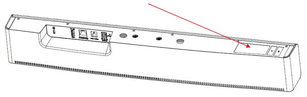
The label shown shall be permanently affixed at a conspicuous location on the device and be readily visible to the user at the time purchase (Labeling requirements per 2.925)
