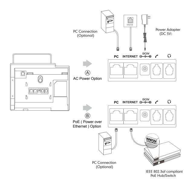
Note: If inline power (PoE) is provided, you don't need to connect the power adapter. Make sure the hub/switch is PoE-compliant.
