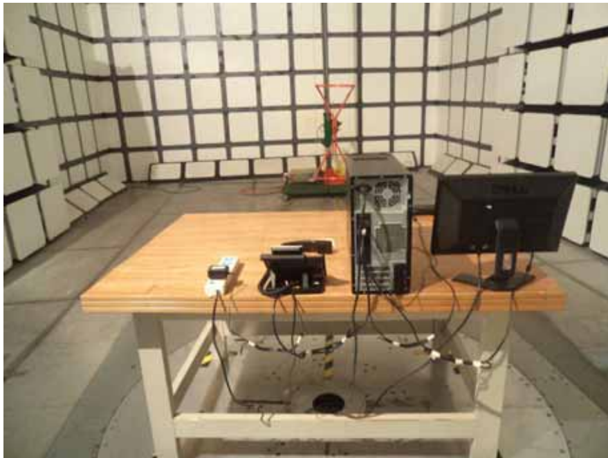
Radiated Emissions – Rear View (Below 1 GHz, for adapter 2)
