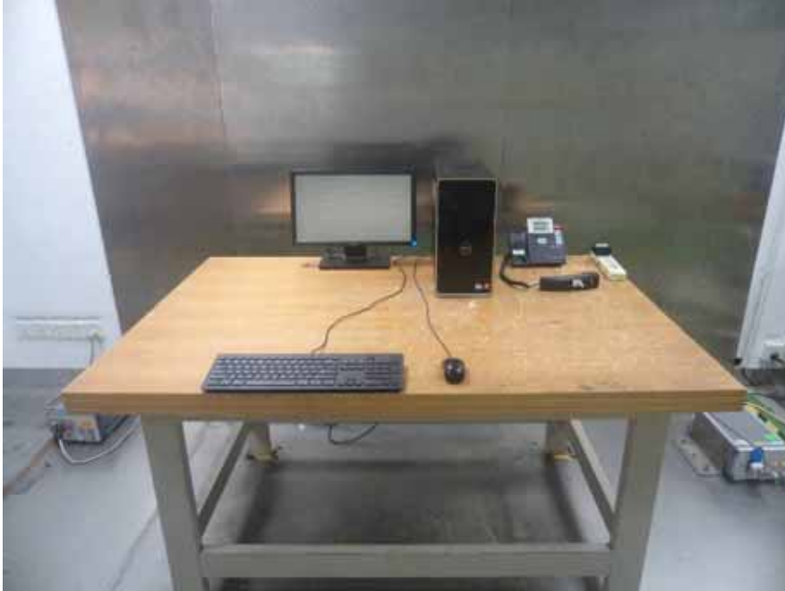
Conducted Emissions - Front View (for adapter 2)
