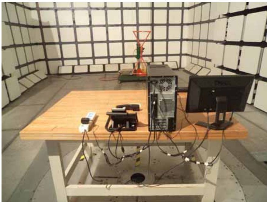
Radiated Emissions – Rear View (Below 1 GHz, for adapter 1)
