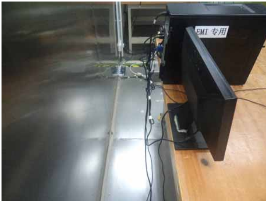
Conducted Emissions - Side View (for adapter 1)
