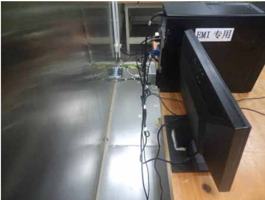
Conducted Emissions - Side View (for adapter 2)
