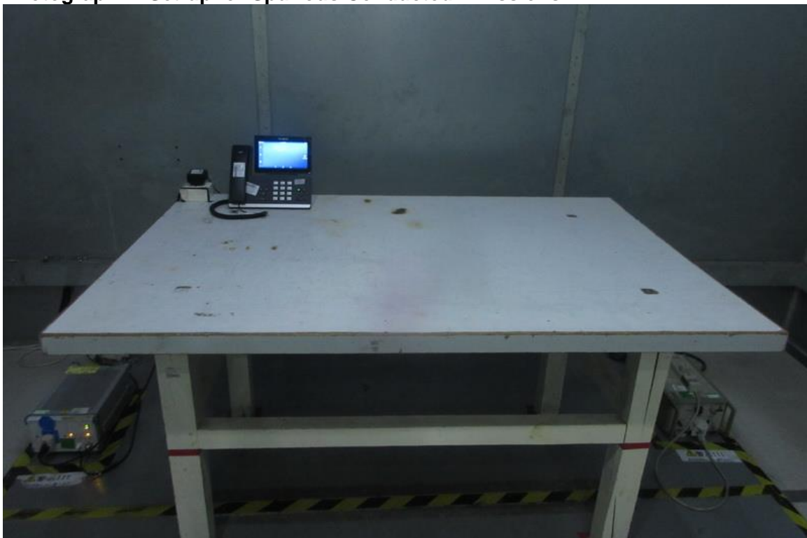
Photograph 4: Set-up for Spurious Conducted Emissions
