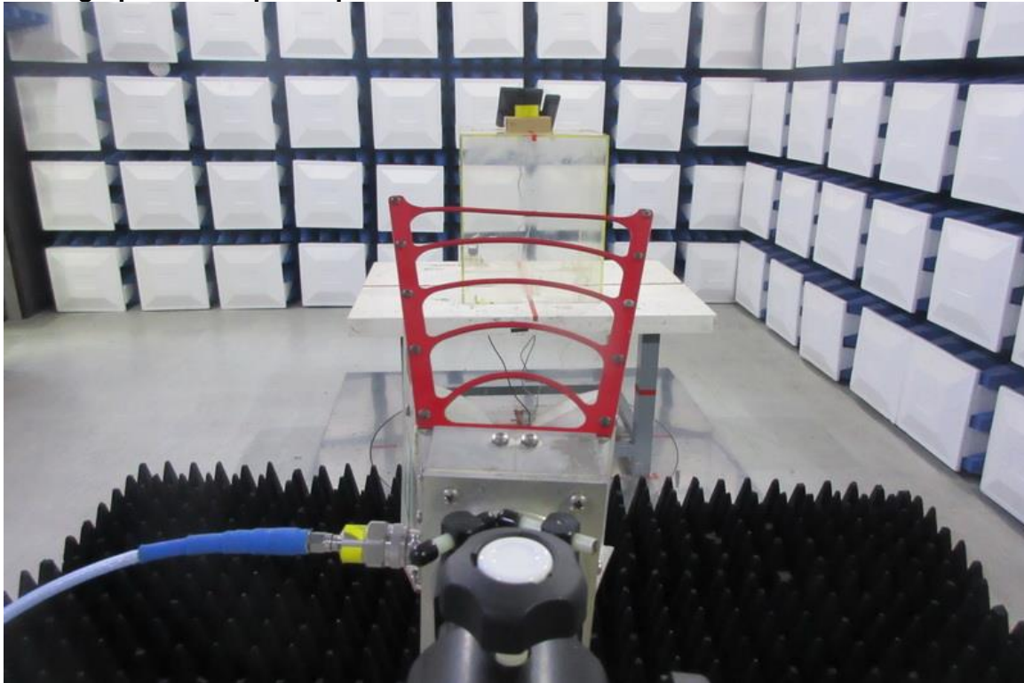
Photograph 4: Set-up for Spurious Conducted Emissions
