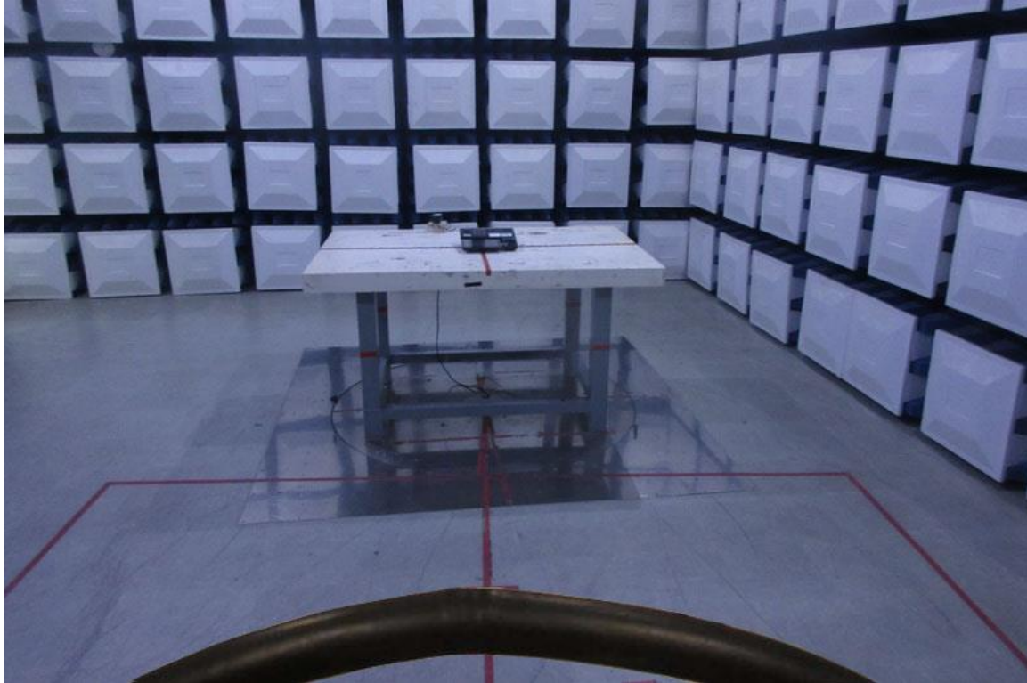
Photograph 2: Set-up for Spurious Emissions for 30 - 1000MHz
