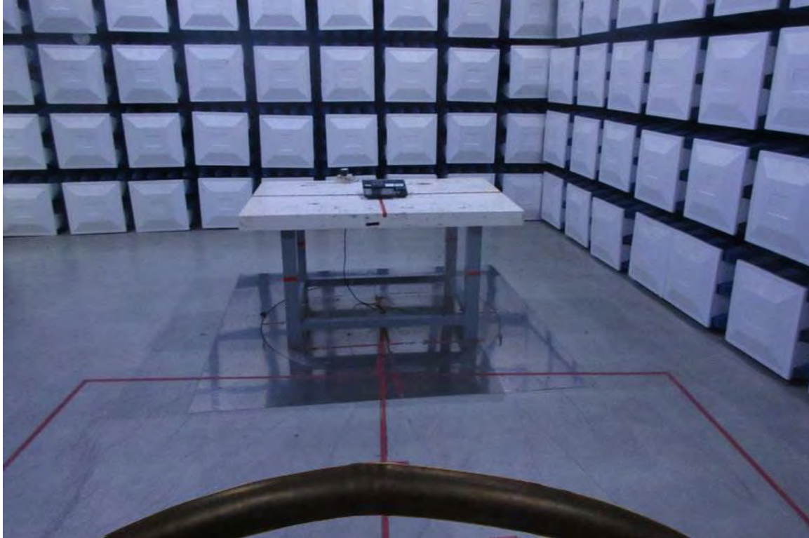
Photograph 2: Set-up for Spurious Emissions for 30 - 1000MHz
