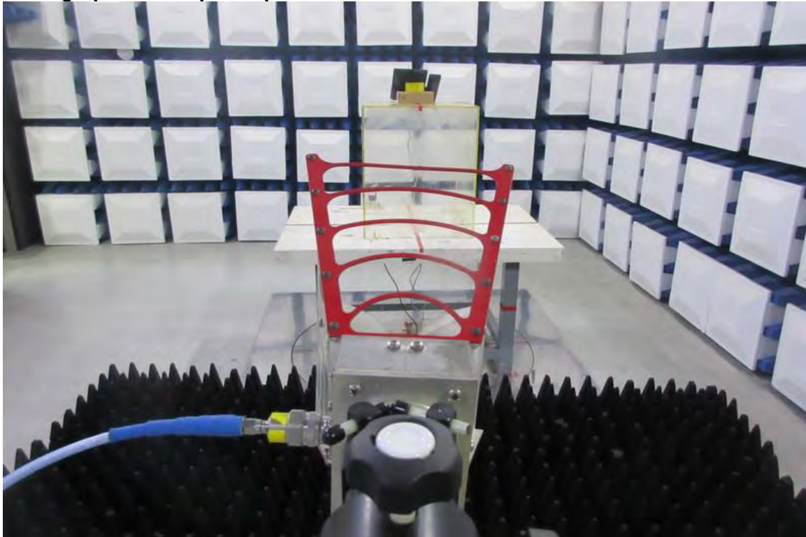
Photograph 4: Set-up for Spurious Conducted Emissions
