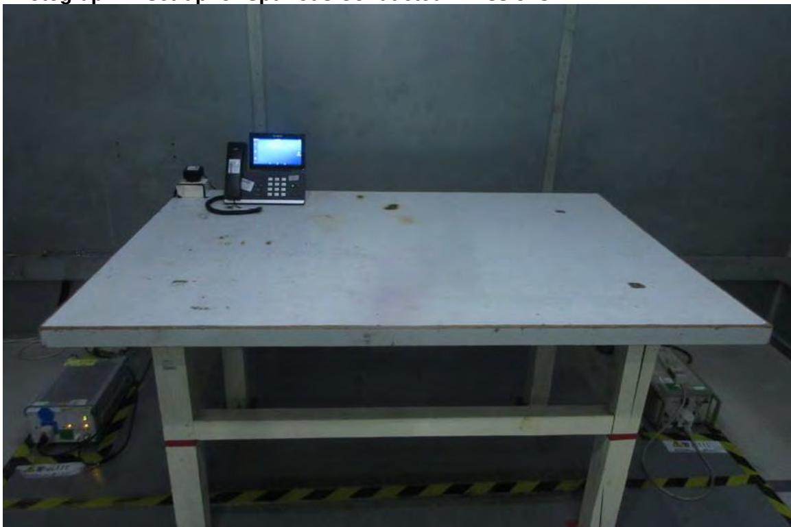
Photograph 4: Set-up for Spurious Conducted Emissions
