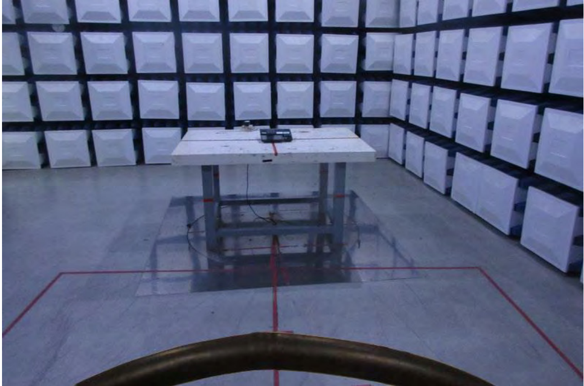
Photograph 2: Set-up for Spurious Emissions for 30 - 1000MHz
