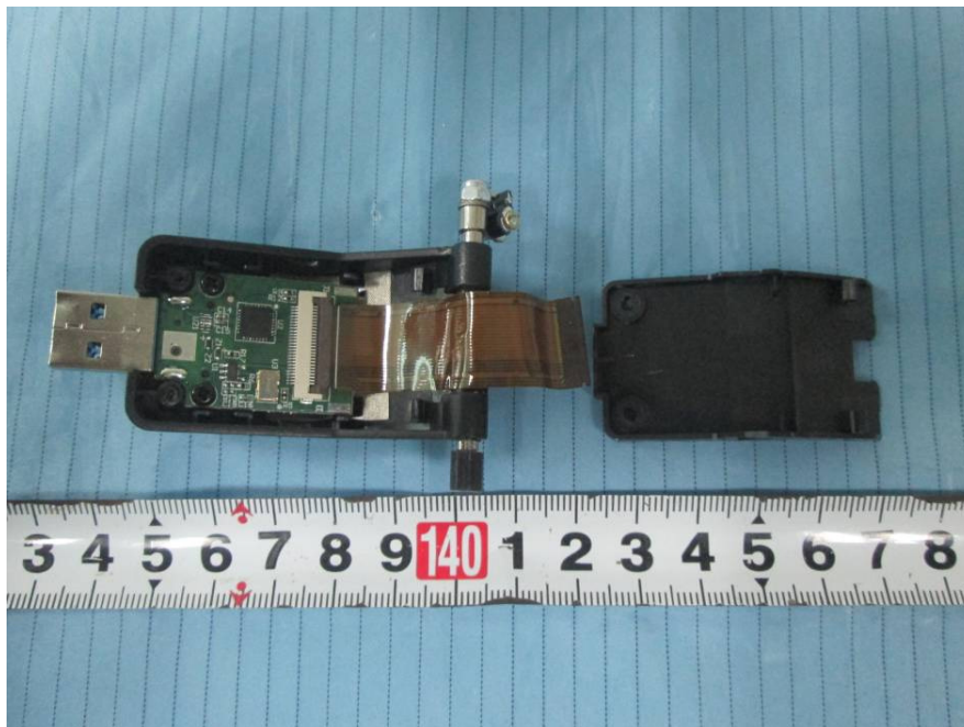
EUT –Camera Cover off View 2
