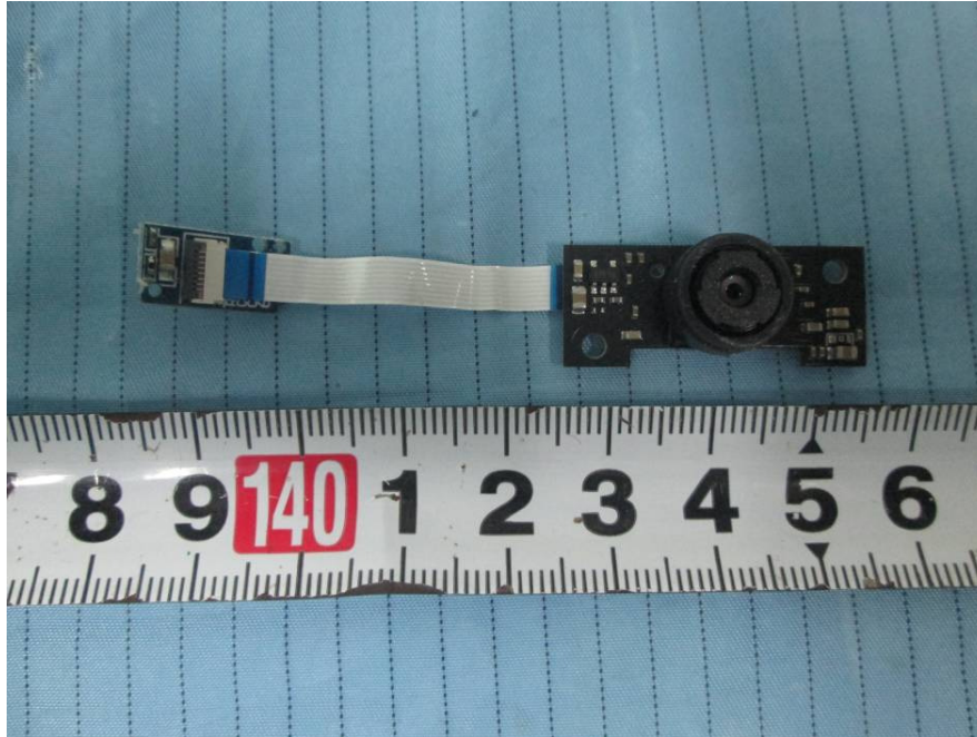
EUT –Camera Main Board2 Top View
