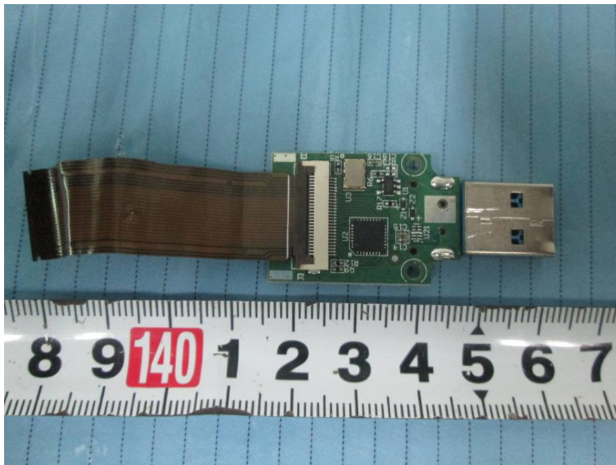
EUT –Camera Main Board 1 Bottom View
