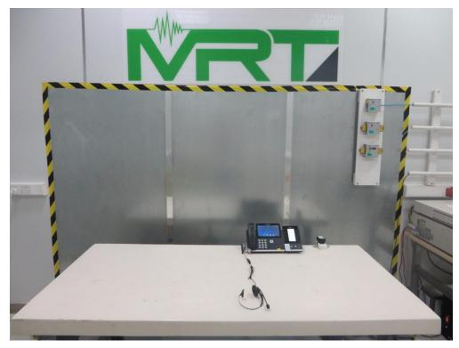
Test Mode 1: Power by adapter and Communication with another IP Phone Description: Back View of Conducted Emission
