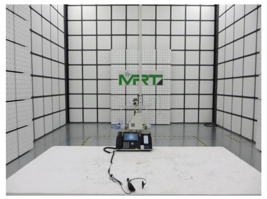
Test Mode 2: Power by POE and Communication with another IP Phone Description: Radiated disturbance Test Setup for 1GHz ~ 18GHz
