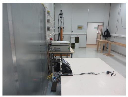
Test Mode 1: Power by adapter and Communication with another IP Phone Description: Radiated disturbance Test Setup for 30MHz ~ 1GHz
