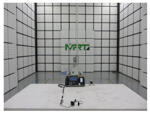
Test Mode 1: Power by adapter and Communication with another IP Phone Description: Radiated disturbance Test Setup for 1GHz ~ 18GHz
