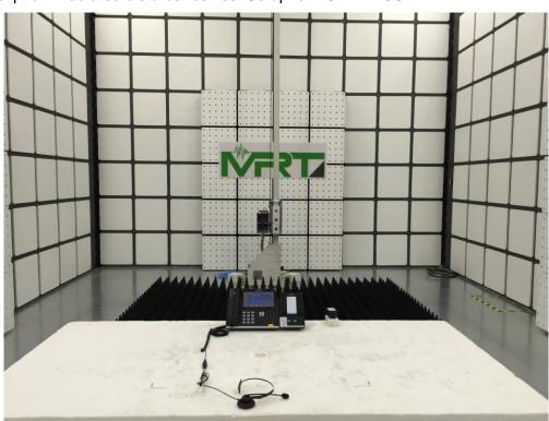
Test Mode 2: Power by POE and Communication with another IP Phone Description: Radiated disturbance Test Setup for 30MHz ~ 1GHz
