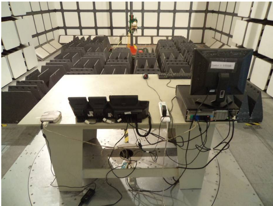
Above 1 GHz: Radiated Disturbance - Rear View (Adapter 2 power supply)
