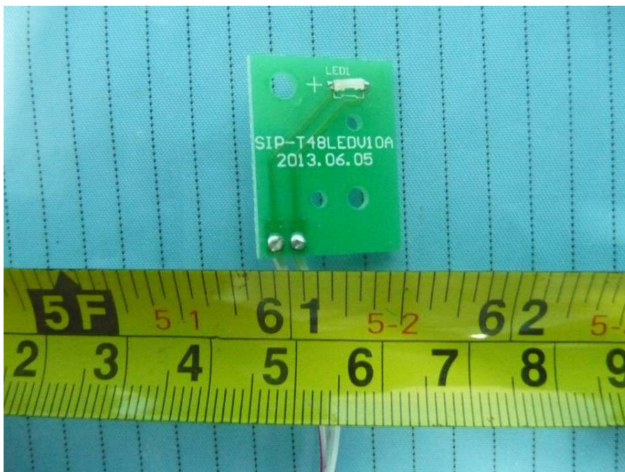
EUT – LED Board Top View
