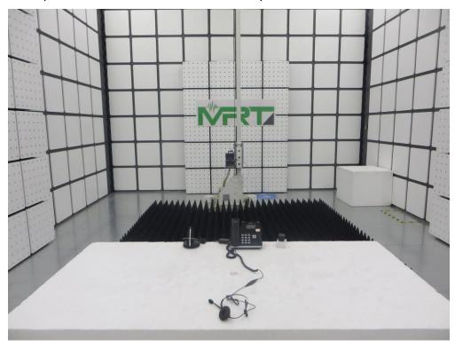
Test Mode 3  $\label{eq:Description:Radiated disturbance Test Setup for 30MHz $$\sim 1GHz$ }$
