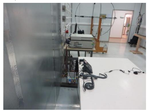
Test Mode 1 Description: Radiated disturbance Test Setup for 30MHz  $\sim$  1GHz
