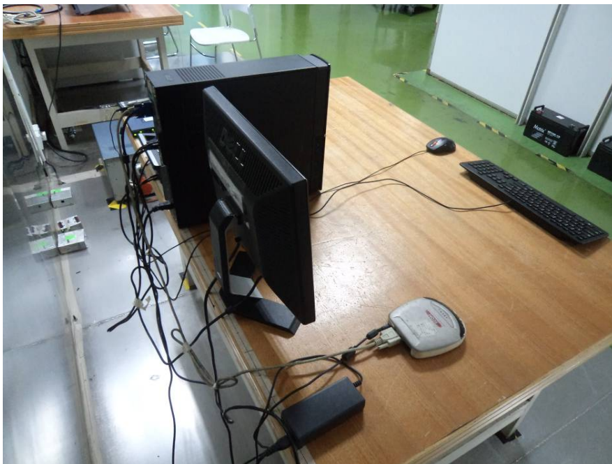
Conducted Emissions - Side View (Powered by PoE)
