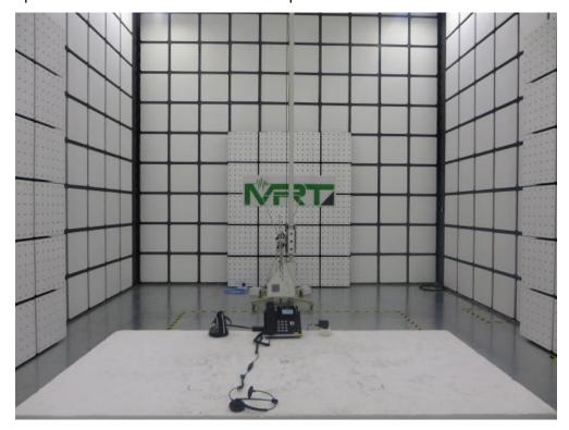
Test Mode 2: Power by adapter #2 and Communication with another IP Phone Description: Radiated disturbance Test Setup for 1GHz ~ 18GHz
