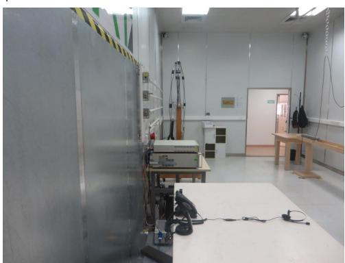
Test Mode 1: Power by adapter #1 and Communication with another IP Phone Description: Radiated disturbance Test Setup for 30MHz ~ 1GHz
