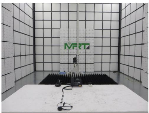
Test Mode 3: Power by POE and Communication with another IP Phone Description: Radiated disturbance Test Setup for 30MHz ~ 1GHz
