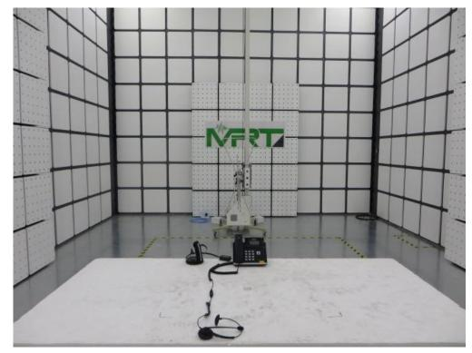
Test Mode 3: Power by POE and Communication with another IP Phone Description: Radiated disturbance Test Setup for 1GHz ~ 18GHz
