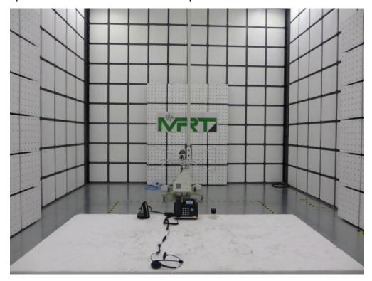
Test Mode 1: Power by adapter #1 and Communication with another IP Phone Description: Radiated disturbance Test Setup for 1GHz ~ 18GHz
