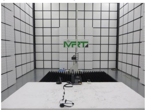
Test Mode 2: Power by adapter #2 and Communication with another IP Phone Description: Radiated disturbance Test Setup for 30MHz ~ 1GHz
