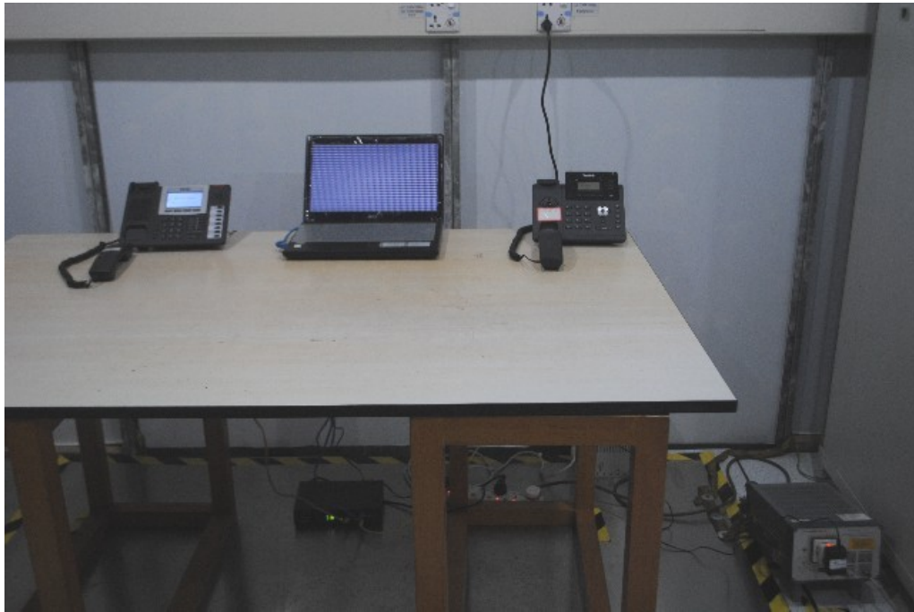
Conducted emission test view –Power Port
