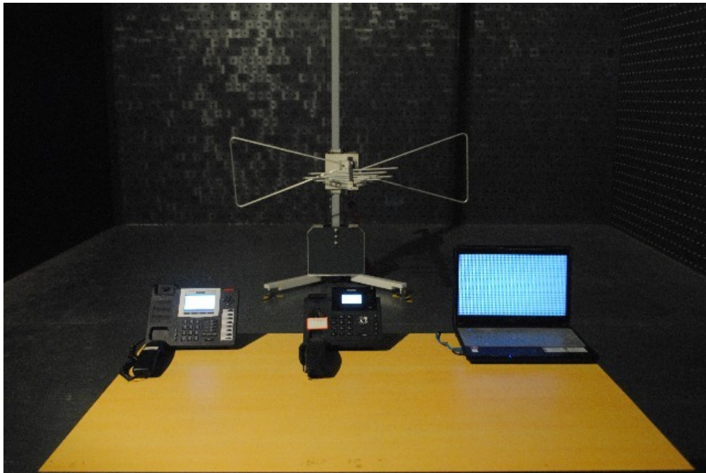
Radiated emission test view (30MHz~1GHz)
