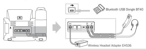
Note: The headset, Bluetooth USB dongle BT40 and wireless headset adapter EHS36 should be purchased separately. The EXT port can also be used to connect the expansion module EXP38 or EXP39. For more information on how to use the EHS36, EXP38, EXP39 and BT40, refer to Yealink EHS36 User Guide, Yealink EXP38 and EXP39 User Guide and Yealink Bluetooth USB Dongle BT40 User Guide.
