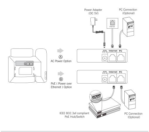
Note: PoE is applicable to the SIP-T23P & T23G IP phones. If inline power (PoE) is provided, you do not need to connect the power adapter. Make sure the hub/switch is PoE-compliant.
