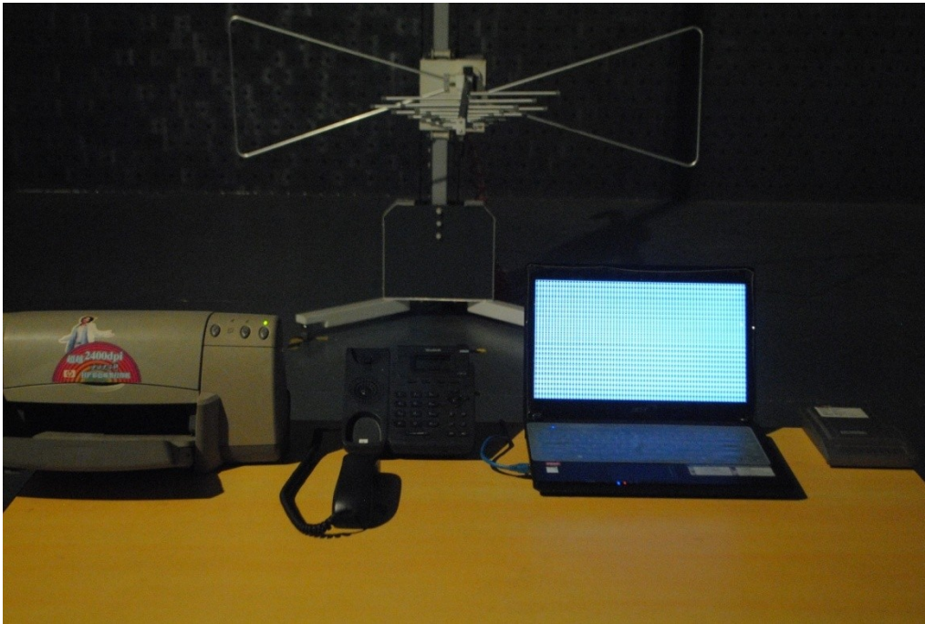
Radiated Emission test view (Frequency above 1GHz)
