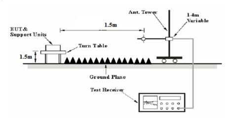
The radiated emission tests were performed in the 3 meters chamber test site, using the setup accordance with the ANSI C63.10-2013. The specification used was FCC 15.209, FCC 15.407, RSS-247, RSS-Gen limits.
