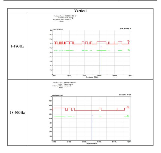
**Worst Test plots for Band Edge Measurements (Radiated)**
