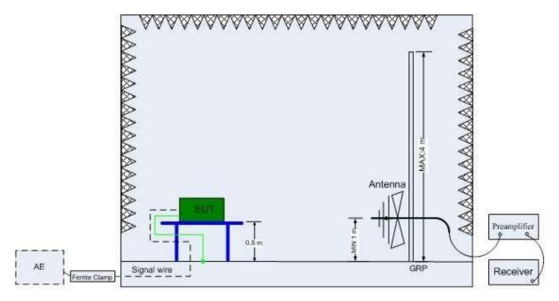
Radiated tests above 1GHz
