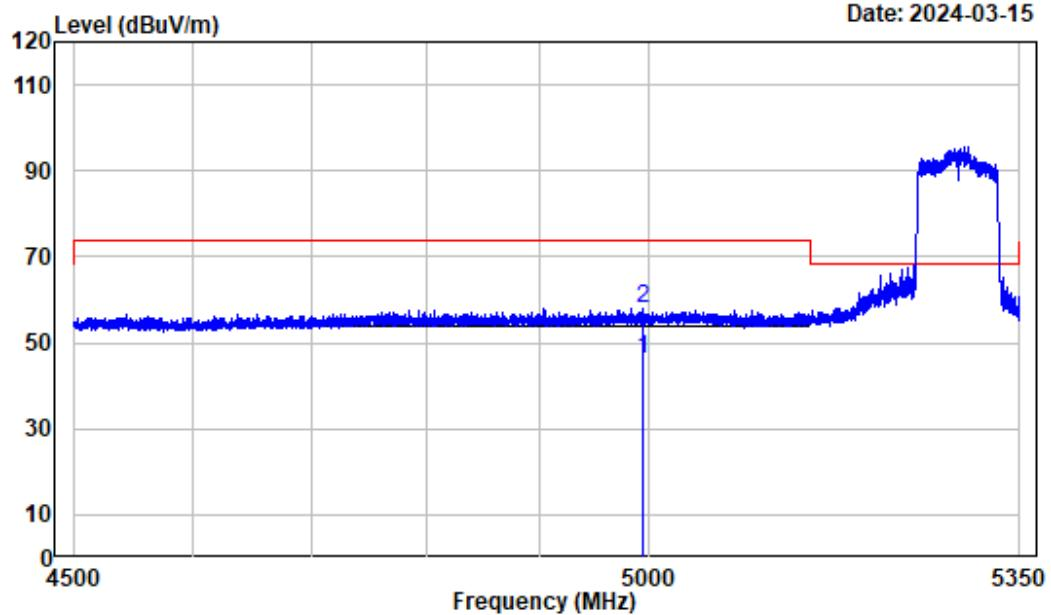
**802.11ac80**Test Channel: **5290MHz**      Ant. Polar. : **Horizontal**
