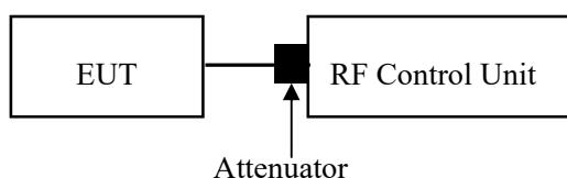
Note: the power meter was integrated in the RF control Unit.
