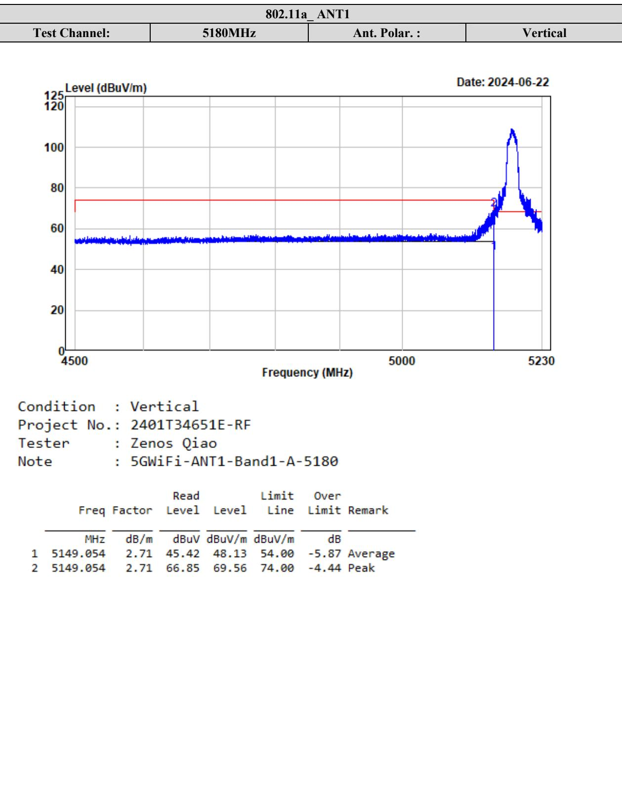
**Test plots for Harmonic and Emissions Measurements: (802.11a, ANT1, 5180MHz)**
