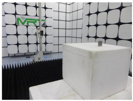
Description: Radiated Power Test Setup for 1GHz ~ 18GHz
