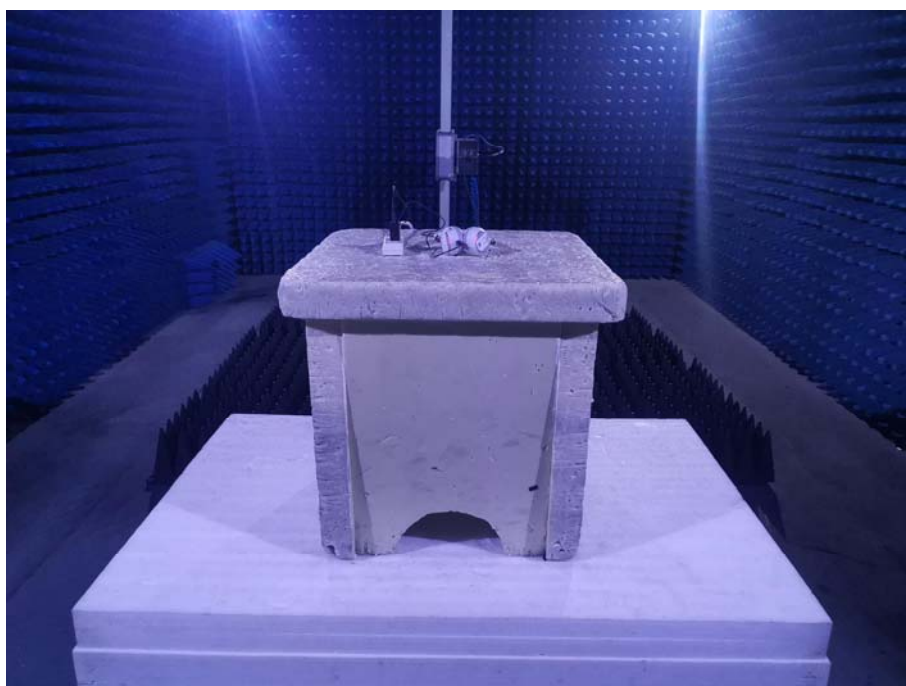
Photo of Radiated Emission Measurement (Above 1G)
