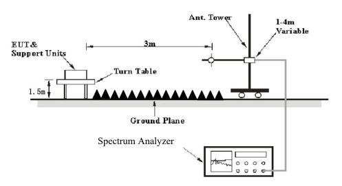
The radiated emission performed in the 3 meters, using the setup accordance with the ANSI C63.10-2013. The specification used was the FCC 15.209, FCC 15.247, RSS-247, RSS-Gen limits.
