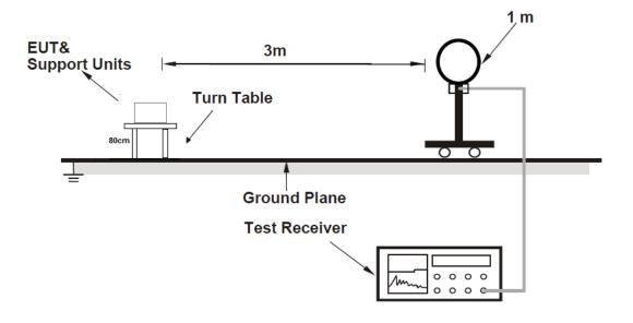
For Radiated emission between 30MHz~1000MHz
