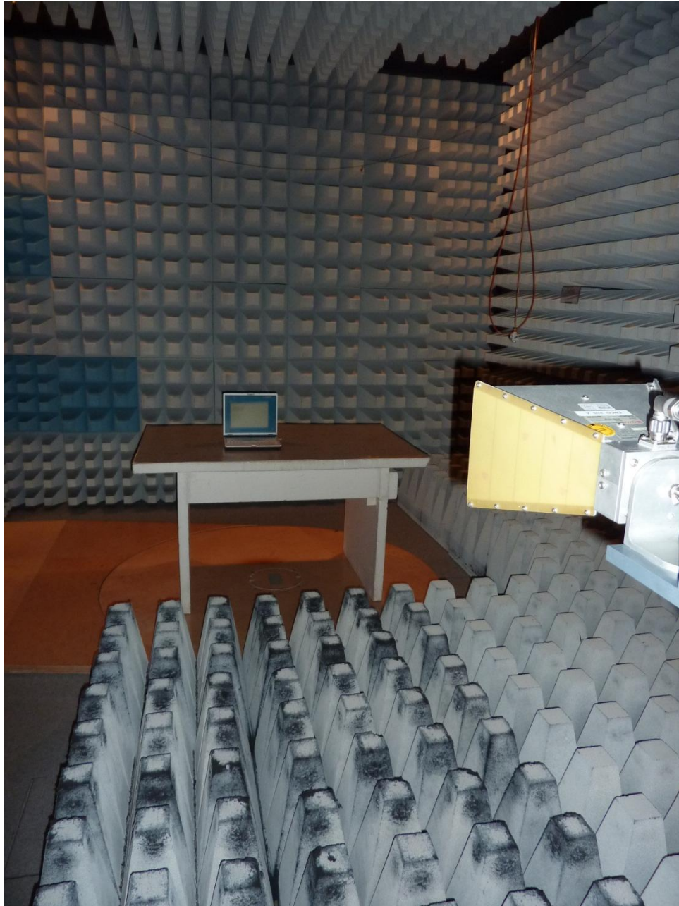
125162_14.JPG: Test setup fully anechoic chamber
