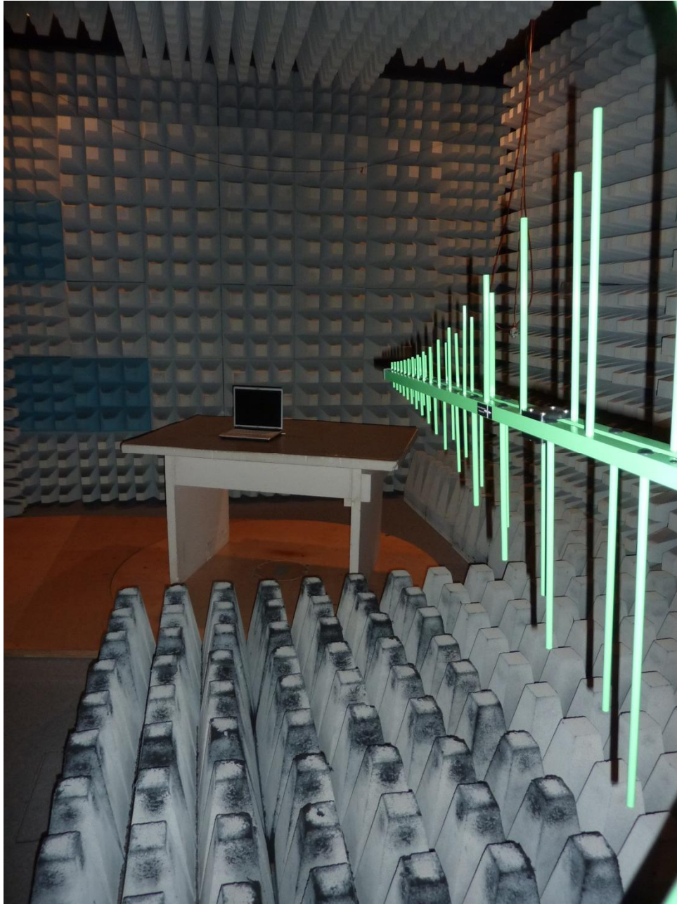
125162_13.JPG: Test setup fully anechoic chamber
